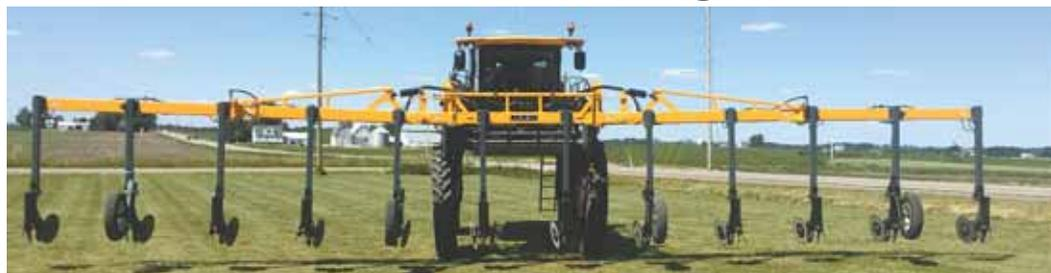
John Miller says his N-Place liquid and dry fertilizer applicator delivers fertilizer to 2 rows at a time. It mounts on any toolbar, including those for high clearance applicators.
