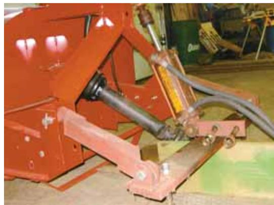
Home-built 3-pt. hitch pins onto snowblower's factory 3-pt. brackets. Lower "push arms" bolt onto a steel plate that fits under tractor's drawbar.
