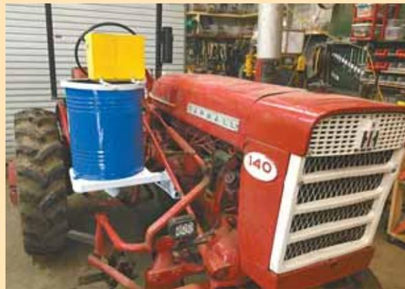
One-row, battery-operated granular fertilizer applicator on Farmall fertilizes garden crops, while a seed trench is dug at the same time.
