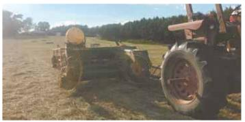
Add-on rake wheels mount on either side of baler pickup.
