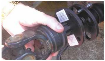
Flat interlocking plate comes in 2 pieces: a male piece with studs that locks onto implement's pto shaft, and a female piece with oblong holes that locks onto tractor's shaft.
