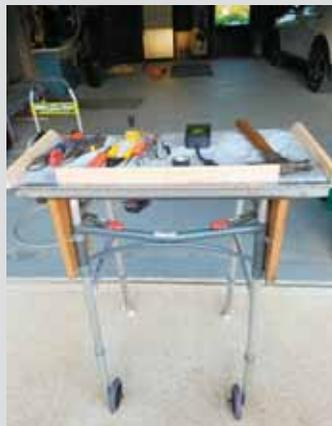
**John Stuber, DeSoto, Mo.:** "I turned a rolling walker into a handy, portable workbench. It's sturdy, lightweight, easy to maneuver, and quickly folds up for storage. I used a piece of scrap aluminum to make the 16 by 24-in. top and screwed wooden pieces onto 3 sides to contain the tools. A piano hinge off an old aluminum cabinet is screwed onto the back side, which allows the walker to fold.
