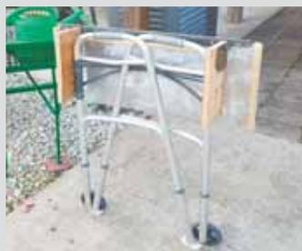
"A pair of short 1 by 6 boards connect the piano hinge to the walker's tubular frame. The boards attach to the piano hinge with hex head screws and to the walker with carriage bolts. A metal strip is screwed onto the piano hinge for extra strength.
