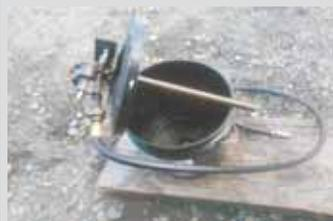
bucket to fill the transmission takes a long time, so I developed a system that uses a cordless impact wrench to do the job. I mounted the oil pump off a Chevrolet car on the bucket lid and run the pump's pickup tube down into the bucket to pump the oil into the transmission."
