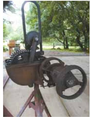
**American Windmill specializes in restoring gear cases to prevent leaks, using a special oil seal and roller bearings.**
