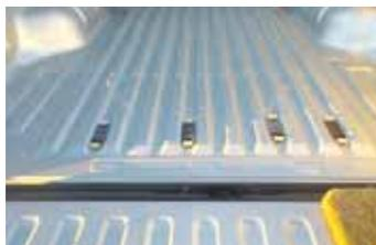
A piece of plywood goes over the four RollBedder dollies that are placed in pickup bed grooves.
