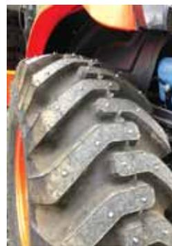
**Screw-On Grip Studs are made from tempered steel, with a welded tungsten carbide rod as the contact point. They can be used on everything from boots to tires.**
