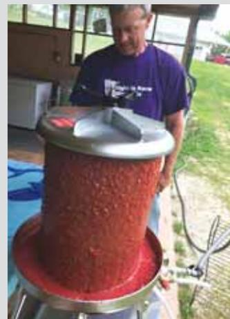
**Jim Riddle uses his Hydropress to turn fresh fruit into juice. "It works faster than steaming and does a better job, and doesn't require any power other than a garden hose," he says.**
