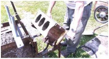
Olson pulls a lever to retract cement block core, then tilts the block out, picks it up with a board, and sets it aside to cure.
