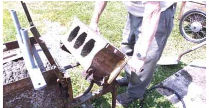
Olson pulls a lever to retract cement block core, then tilts the block out, picks it up with a board, and sets it aside to cure.
