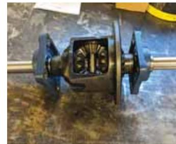
plates out of 3/8-in. flat stock for end caps on the pipe and drilled holes for the shafts.
