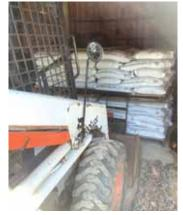
Convex mirrors are designed to mount on both sides of skid loader.
