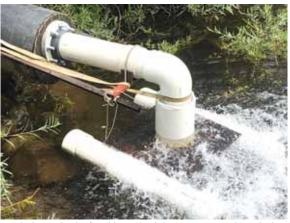
**PVC** float system is made from 2 parts - a 90-degree elbow with a 6 by 8-in. bushing on the bottom, H-shaped float with a 6-in., centervertical cap.
