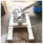
As float rises with the water level, the vertical cap puts pressure on bushing to seal off a pond inlet pipe.
