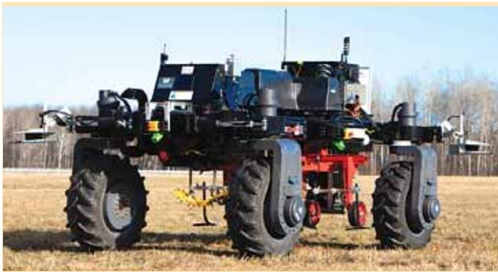
All-electric autonomous Erion tractor comes with 9 electric motors with gearboxes. Each wheel has a drive motor as well as a motor for steering. The ninth motor raises and lowers undercarriage tools, such as a cultivator.
