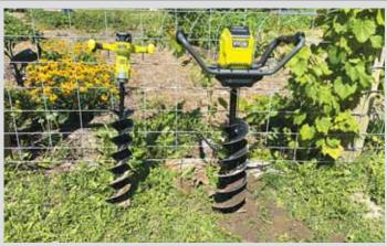
"With the Ryobi cordless, kickback is not a problem. Hit a rock or buried metal and it stops and resets so you can reverse it out of the hole."
