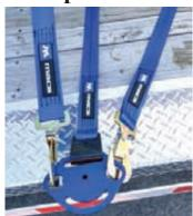
The Monkey Face fits into a 1 1/4 in. stake pocket and is secured with a cotter pin. The top plate can accomodate various hooks, strans or chains.
