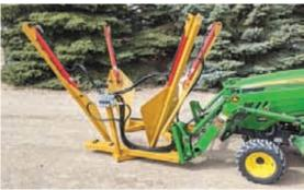
Klassen developed a hydraulic tree spade for use with his compact tractor that costs far less than larger models commercially available.
