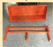
Mattiuz's "shorty forks" use two friction eyebolts at each end to attach to the tractor bucket.
