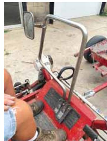
An old handrail from a semi-tractor formed into a new shape makes a great rearview mirror bracket and handrail on Al Hernke's zero-turn mower.
