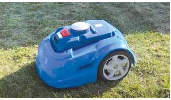
The M1 can mow about an acre in 6 hrs. on a single full charge of the swappable battery.
