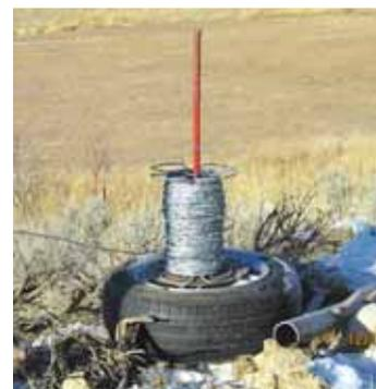
**Thomas built a fence wire unroller using a small car tire and rim with a metal plate and rod.**
