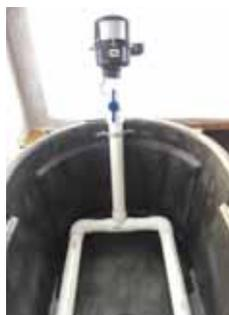
**Wash station uses a 100-gal. stock tank with a 1 hp. blower to move air through PVC lined with holes.**
