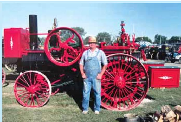
Scott Wiley had an authentic flywheel made to original specifications for his 1902 Robinson steam engine. The design was re-created from a photograph using computer software.
