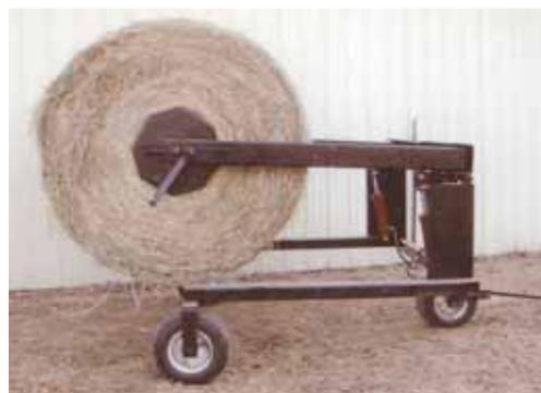
Tag-along cart (left) grabs round bales and lifts them off the ground. A hand crank is used to spin bale. Skid loader-mounted spinner uses a hydraulic motor with a chain drive.
