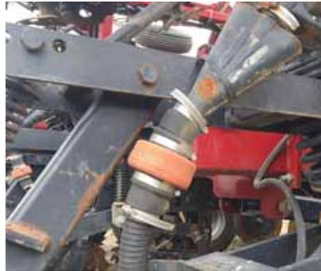
Wireless blockage sensor sends out radio signals, powered by a built-in medical grade lithium battery.
