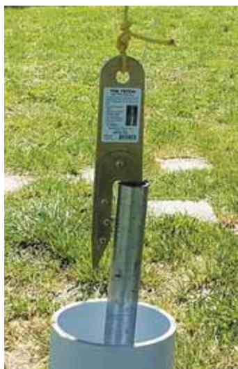
When lowered down through a pipe via a retrieval line, one of The Fetch jaws slides into the opening of the broken pipe and grabs it there, while the other grips it on the outside.
