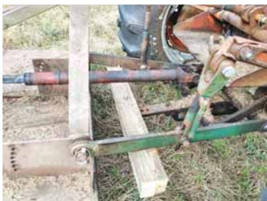
Smith says the weight of the rotary mower holds the 4 by 4 in place. When he wants to detach the mower, he simply lifts it up and unbolts the 4 by 4.
