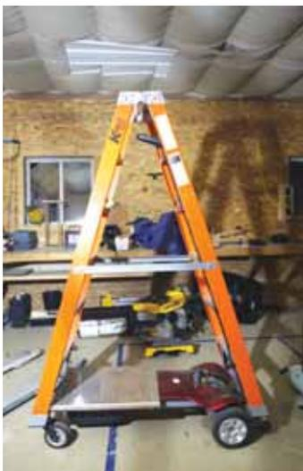
Rolling ladder is a 6-ft. step ladder welded to a motorized scooter with the seat removed and is operated by a joystick on the ladder.
