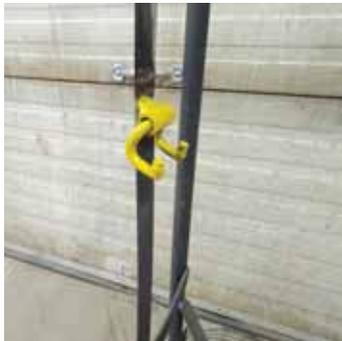
"The hook is made from a 9-in. piece of 5/16-in. rod and a 1-in. piece of pipe with a matching center hole," explains McLaen. "It took about 30 min. to build and paint. It makes moving the heavy garbage containers a breeze."
