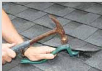
**Roof Snake:** Replacing a 3-tab shingle without damaging the surrounding shingles isn't easy. The Roof Snake has a claw on one end for pulling nails and an offset nail slot at the other end that lets you pound in a nail under the roofing tab without having to bend it back all the way. Sells for \$30-40 at retailers and online ([www.pactool.us](http://www.pactool.us)).
