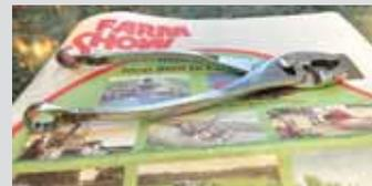
**Jim Rankin, Paris, Ky.:** "I weld a 1/2-in. box-end wrench on one handle of a set of pliers and a 9/16-in. wrench on the other handle. It makes my pliers about the handiest tool I own. I've used this idea for many years and whenever the pliers wear out, I just go to the shop and cut off the ends of a couple of wrenches and weld them to the pliers. They're quite a conversation piece."
