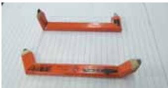
"I took 2 ordinary carpenter's pencils and cut the ends off with my miter saw," says McLaen. "Then I glued them back together at various 90 and 60-degree angles to the original pencils. They cost me less than a buck each and make marking a lot easier."
