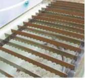
Merrigan inserted blades with their cutting edges down into slots in an angle iron frame to form table's working surface.
