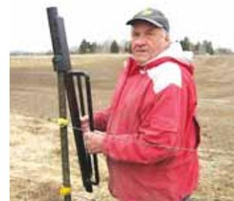
Ron Lanser is shown using Momper’s post driver. Top of post slides up and down inside the angle iron, driven by the solid steel shaft at the top.
