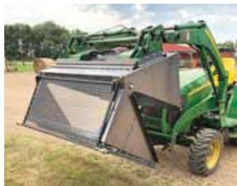
**Burn Bucket mounts in place of a front-end loader bucket and is designed with a clam shell dump.**
