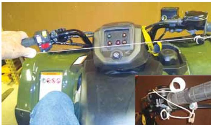
**Henderson used a clamp, pulley and nylon cord to control the throttle on his Honda ATV with his left hand. A small piece of pvc that fits over his thumb.**
