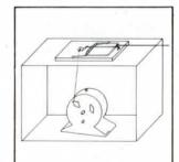
A length of plain wire or strong cord is connected from the engine's cut-off switch to the swinging guillotine arm of the trap. When the trap snaps, it pulls the switch to shut off the engine. You simply set the alarm clock to ring at whatever time you want the engine or motor to shut down.
