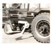
roller chain connects the seatleveling shaft and sprocket to the gear hox
