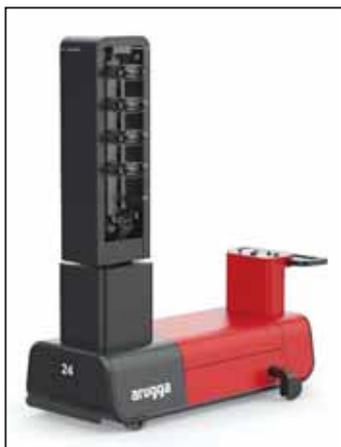
**Pollination robot has cameras to determine when to use air pressure to shake pollen loose.**
