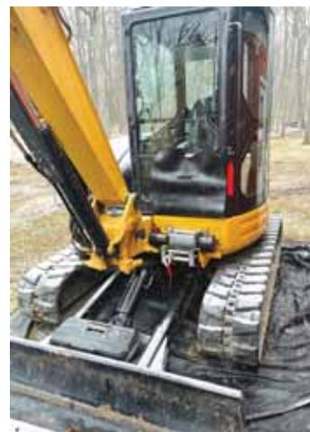
**Yax mounted a winch that rotates with the cab to his mini excavator to clear fallen trees on his property.**
