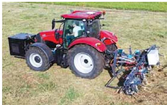
**Distance between rotors is adjustable through actuators which allows operator to optimize for any type of grass.**
