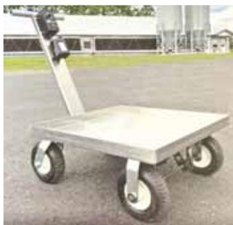
**Cart is made of durable aluminum, has a heavy-duty DC motor, and fits through any door at least 28-in. wide.**
