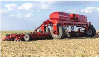
Self-propelled seeder has a centralized motor placed above the planting rows.
