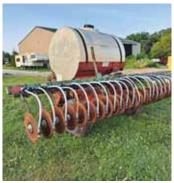
Dykstra plumbed the applicator with pvc pipes and tees above each opener leading to anhydrous drop tubes. He zip-tied the pvc pipe to the toolbar for flexibility as it moved through the field.
