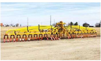
Davis says the bar's uniquely designed flux manifold features a V-shaped bottom to catch debris and rocks without plugging the product lines.
