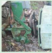
Shaft welded to center of drum bottom have a steel plate housing and two pillow block bearings inside.
