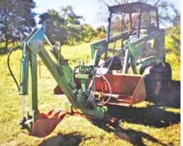
plates are 1/2-in. steel. I may have overdone the strength, but I wanted it to be safe. I welded most of it with 718 rods. It's harder to grind down, but it's better for penetration
