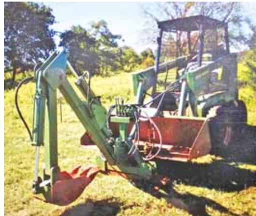
plates are 1/2-in. steel. I may have overdone the strength, but I wanted it to be safe. I welded most of it with 718 rods. It's harder to grind down, but it's better for penetration
