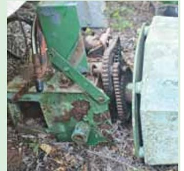
stationary cement mixer. Shaft welded to center of drum bottom have a steel plate housing and two pillow block bearings inside.
