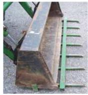
"It works very well to get a bite with the bucket into manure that's packed with straw," Miller says. He also uses it to clean plant debris in the garden and for lifting pipes and 2 by 4s.
