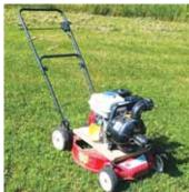
Pacer pump and Honda engine mounted to a mower deck
