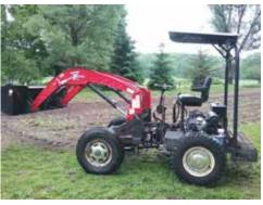
Petersen purchased a hydraulic steering mechanism designed for a Massey Ferguson tractor to control the rams on the articulation.
