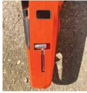
Ryobi and Echo saws both have handy chainsaw tool holder slots.
