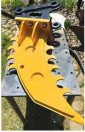
Yax says, "I made the ripper in two parts because I wanted to be able to attach other accessories that I'd like to build. To fit them together easily, I cut a 1-in. hole in the center of the excavator receiver that mates up with a 1-in. post on the ripper."
