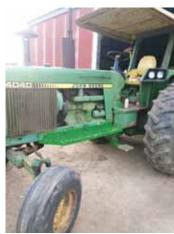
Tractor walkway made from angle iron and safety tread plank.
