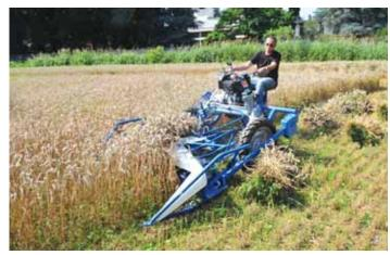
BCS 622 reaper binder has a working width of 55 in. and is available as a motorized cutting bar without binder.
