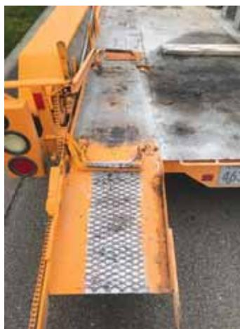
Trailer ramps move up and down when wheels cause activator bars to move and drive sprocket and roller chain.
