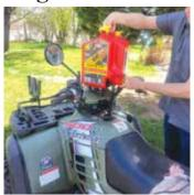
SureCan can be set down on a mower or tractor as the fuel is being dispensed. The flexible nozzle rotates down more than 180 degrees.
