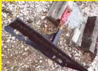
I bought a receiver hitch with a mounting plate to mount on the front of my skid steer. Then I adapted a quick disconnect hitch off an old corn picker and fit that to the receiver hitch. I use this to move equipment around - augers, hay racks, etc. - without having to get off the skid steer. Very useful. (Richard Rosener, Vail, Iowa)
