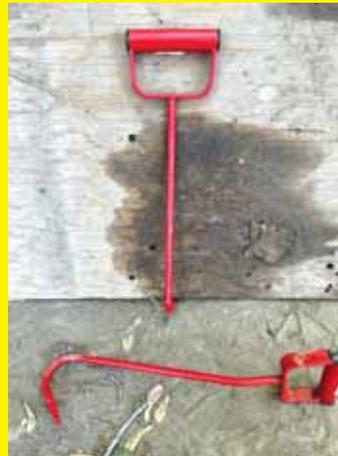
I discovered my hay hooks work great for carting around sheets of plywood by myself. Just reach down to slip the hook under the center of the sheet and you'll be able to handle 3/4-in. plywood with ease. These hooks have a lot of miles on them from stacking thousands of bales above our dairy barn. Now that I have a new use, I can keep putting them to work. (Gary Swensen, Yankton, S.Dak.)
