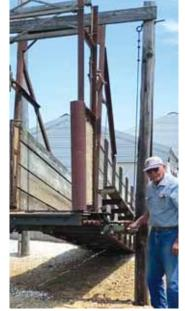
Dennis Backhaus built an adjustable platform on the front of his loading chute that moves side to side and aligns to the door of a livestock trailer.
