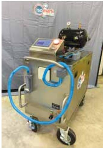
**Battery-powered breathalyzer is able to determine cattle health before symptoms develop.**
