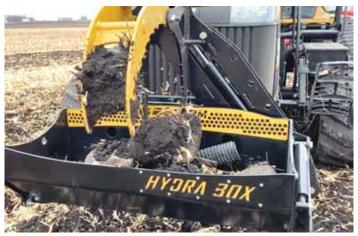
Hydrabox rock picker uses two sets of opposing, grade 80, steel claws with a tensile strength of 80,000 lbs. The 3-in. hydraulic cylinder controls the claws with 31,000 lbs. of pressure.
