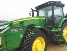
FieldSeal toolboxes are made with 3/16-in. powdercoated steel with a rubber seal like those used in cab and truck doors. The seal makes them fully dust and weatherproof.
