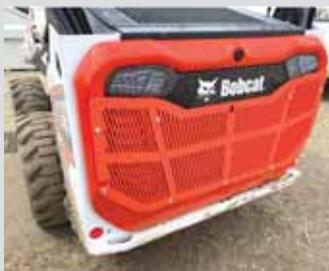
**May Wes Company, Hutchinson, Minn.:** (www.maywes.com; ph. 800-788-6483) "Our rear debris screen for Bobcat skid loaders shields the radiator, helps with overheating, and is made from UV-resistant HDPE. Less expensive than OEM shields and made for ag, landscape and forestry applications, the shield easily installs by drilling and bolting into place. Made in the USA."
