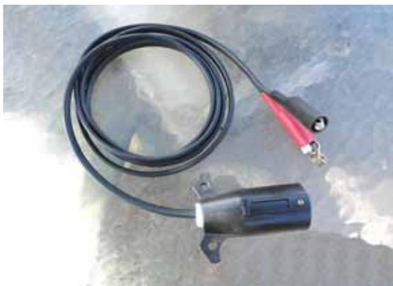
Willett created a power outlet from his pickup hitch connector so he could easily work on his tailgate.
