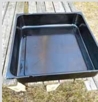
**Mark Yax, Solon, Ohio:** "I had an electric stove that I was tossing out. When removing the bottom drawer, I noticed that the stamped steel tub would make a nice drain pan or parts washing tub. I removed the front door panel and cut off the ears that held it on with my angle grinder. The only other thing I had to do was to weld up some small holes. This should work well for changing the oil in some of my equipment as it holds quite a bit. I will also use it for cleaning some larger parts."
