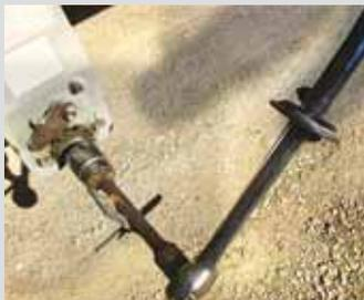
**Tom Hansen, New Hartford, Iowa:** "I welded a socket to a 3/4-in. drive extension and put crossbars on the extension and a big washer on the handle with a hose clamp to keep it all from falling through the grates."
