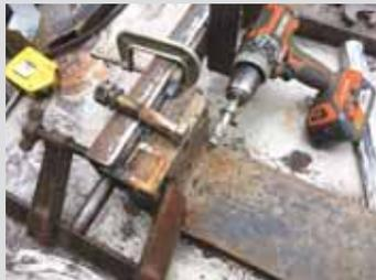
**Jack Griffith, Venus, Texas:** "To center a drill when drilling into a stepped hole, I stack fender washers on the bit that match the diameter of the hole I'm drilling into the bottom of. In this case, I used a stack of nuts to put the washers at the depth I wanted to drill the hole."
