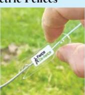
Fence De-Fence tool allows electric fence wire to be moved for easier clearing without being shocked.
