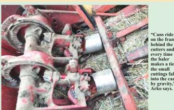
on the frame behind the cutters and every time the baler makes a tie. the small cuttings fall into the cans by gravity," Arko says.
