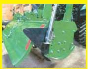
When rototilling beside small plants, dirt would spill out and bury the plants. So, I installed a shield (the black triangle in the photo) to prevent the problem. Worked great. (Garnet Powers, Marsden, Sask.)
