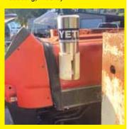
My redneck Yeti cup holder was made from a piece of pvc pipe. I just cut a slit in one side, so it expands to grip tight, and then attached it to the side of the tractor. (Clotfelter Farms, Bogart, Ga.)
