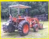
I previously sent you a picture of a heavy wood stove insert that I repurposed as a tractor counterweight by fitting it to my 3-pt. hitch. I've since welded a trailer hitch to the stove, so I have a drawbar again without removing the counterweight. I also fitted the tractor with the roof of a golf cart. (Pete Jordahl, Oswego, N.Y.)
