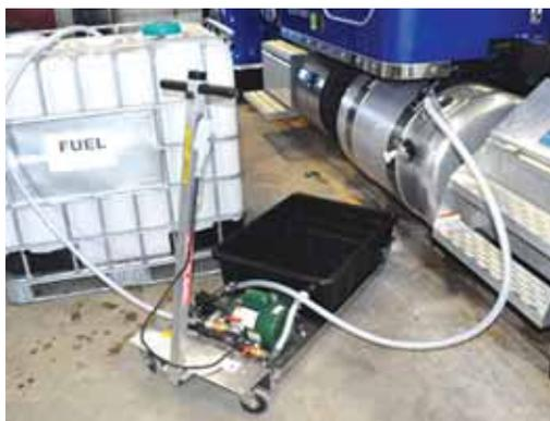
**Oil Kaddee runs off a 115-volt 1/2-hp. motor and includes a 20-in. mesh stainless filter and an 8-ft. discharge hose with all quick tach fittings.**
